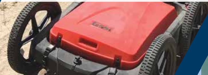
Geology students use ground penetrating radar equipment to survey the subsurface.
