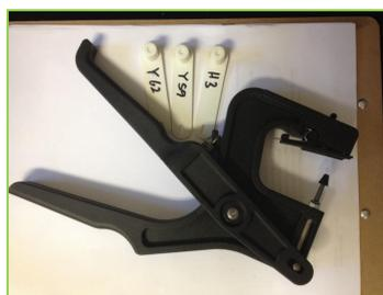
Figure 1: TypiFix™ collector unit and sample wells
