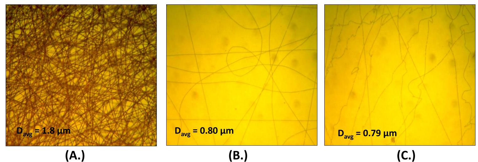
Micro slide images (above) of solution electrospun at (A.) 0%, (B.) 30%, (C.) 50% relative humidity.
