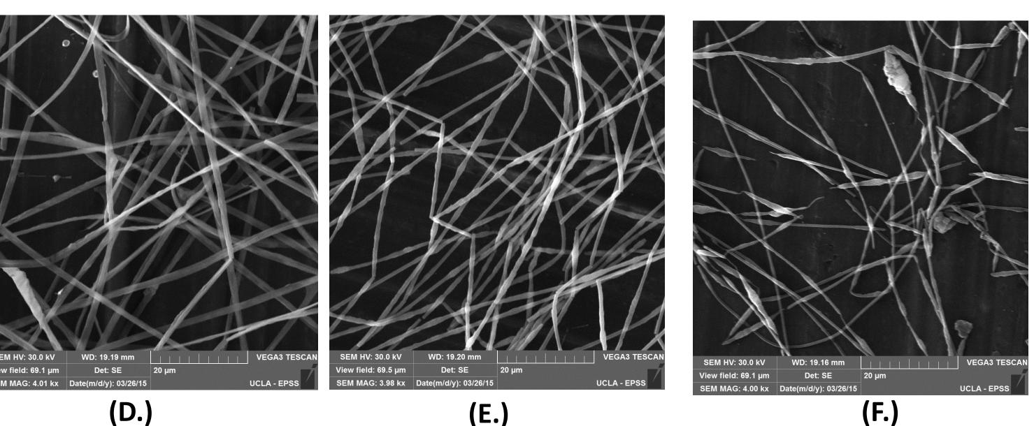
Scanning Electron Microscope images (above) of solution electrospun at (D.) 0%, (E.) 30%, (F.) 50% relative humidity.
