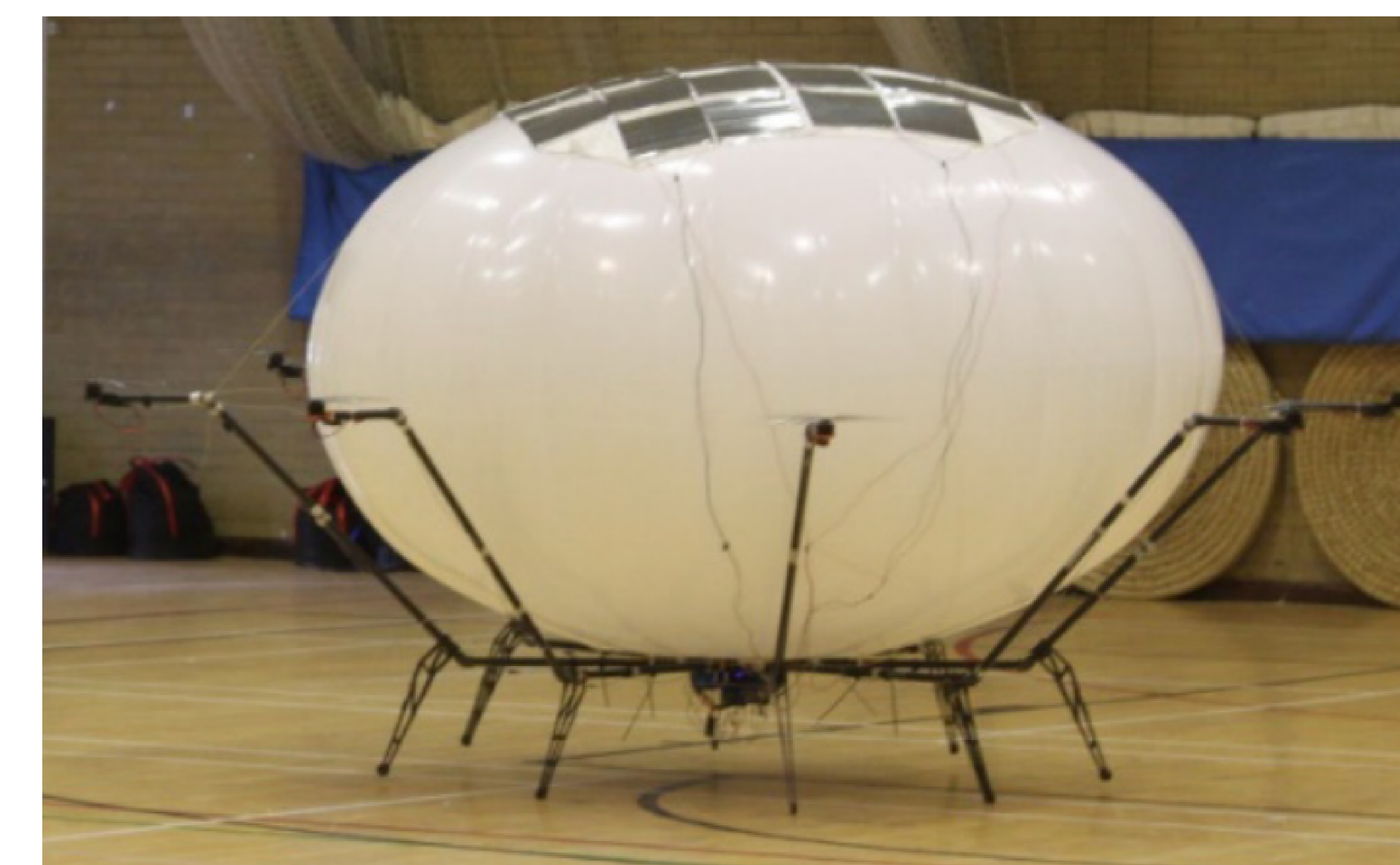
Figure 4: An example of an LTA UAV design with more propellers for control and solar panels mounted on it to lengthen its flight time.
