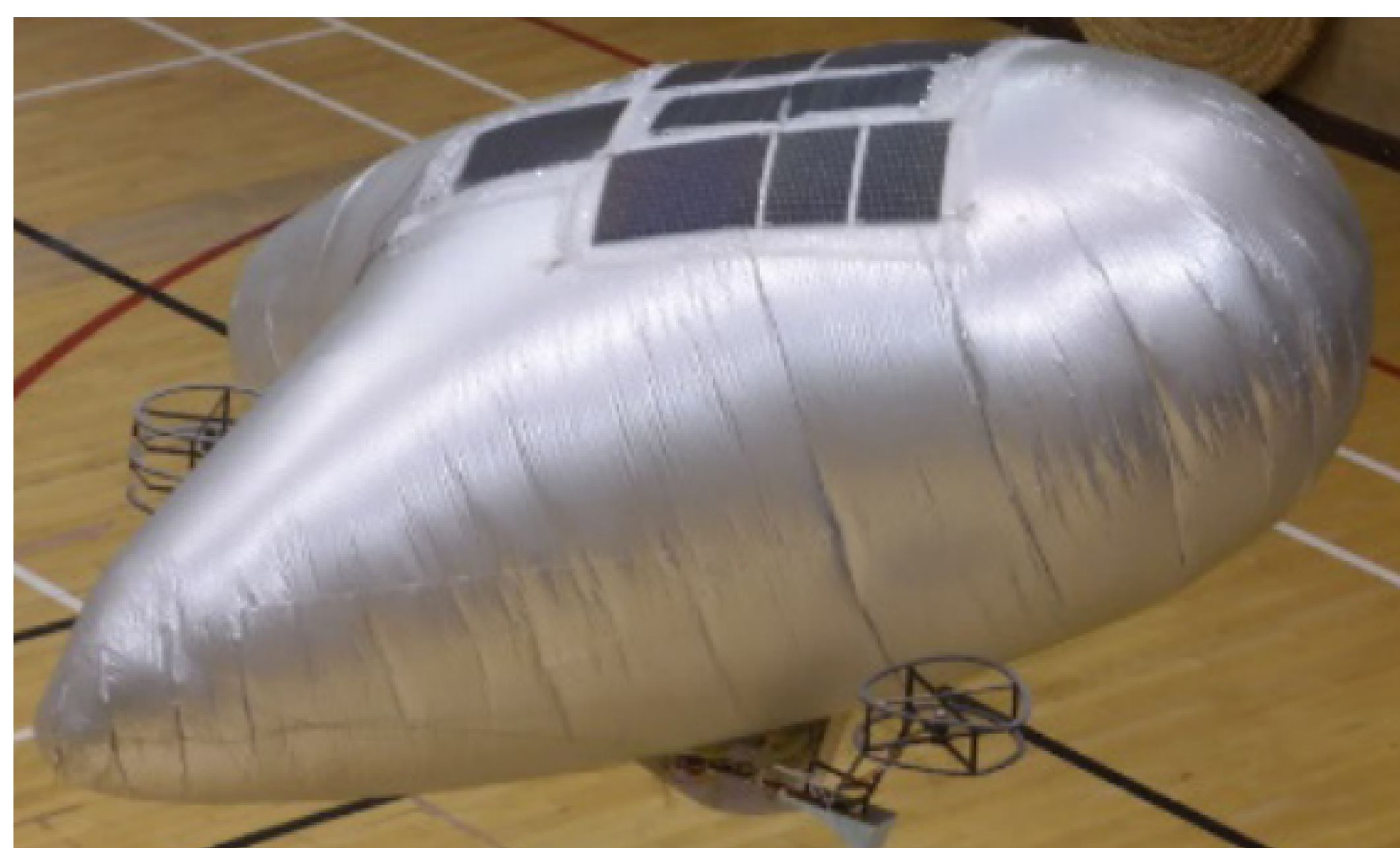
Figure 2: An example of an LTA UAV design with solar panels mounted on it to lengthen its flight time.
