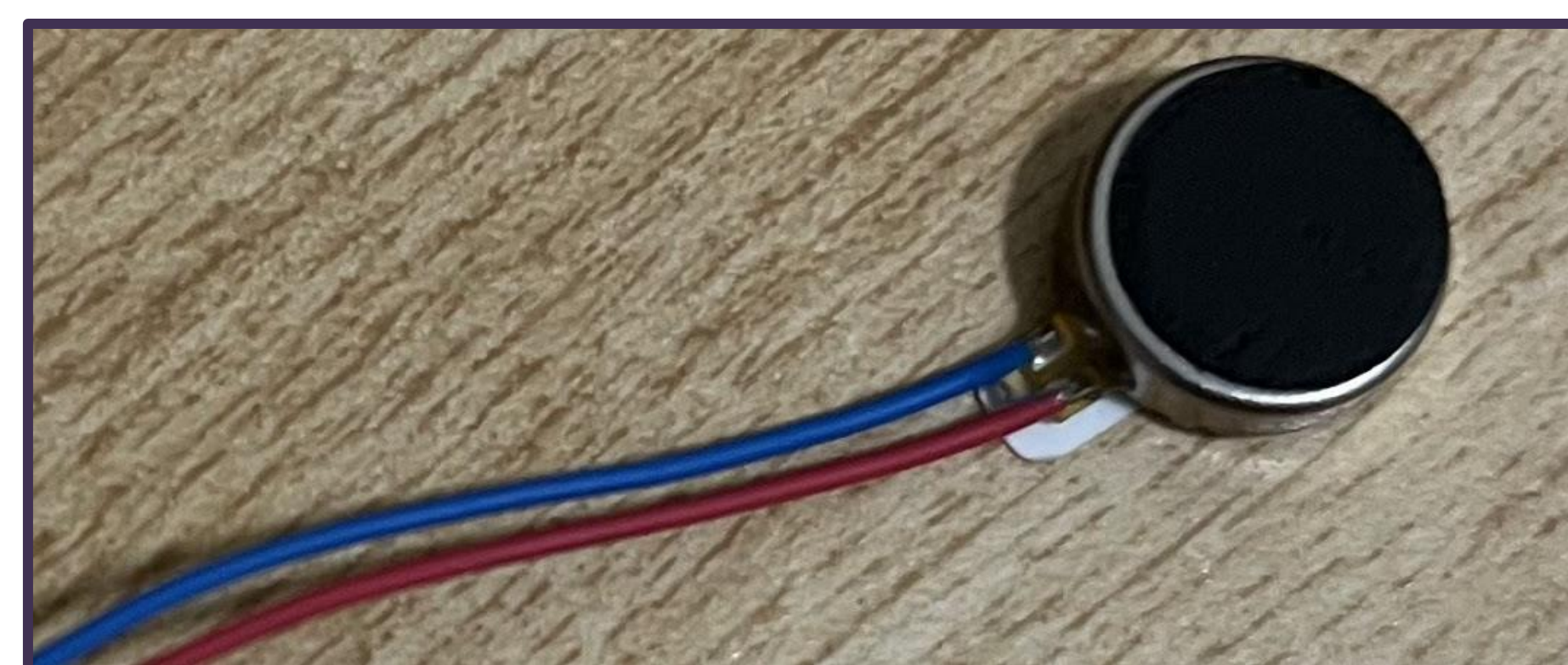
Figure 1: An example of the coin vibration motor used in this project.
