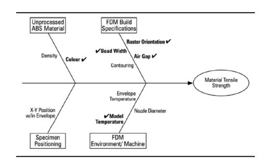
Of the mentioned build parameters, air gap and raster orientation have been shown to have the most significant effect on material properties. Contouring has been shown to have effects on material properties in some cases, but its full effect is not completely understood.
