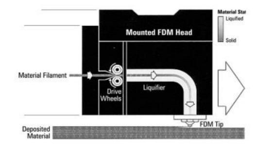
Traditionally, FDM has been used exclusively for the purposes of rapid prototyping due to its low cost, simple setup, and high versatility. That being said, there may be potential for the use of FDM parts in some low-load applications. For designers hoping to use FDM to generate production parts, a thorough understanding of the material properties of FDM-manufactured parts is crucial.
