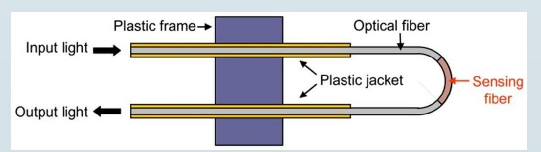
The sensitive region of the optical fiber is freely exposed It is preferable that the sensitive regions has a protective covering that maintains the sensitivity and that can readily accept fluid without disrupting the structure and the shape of the sensor and the compartment.
