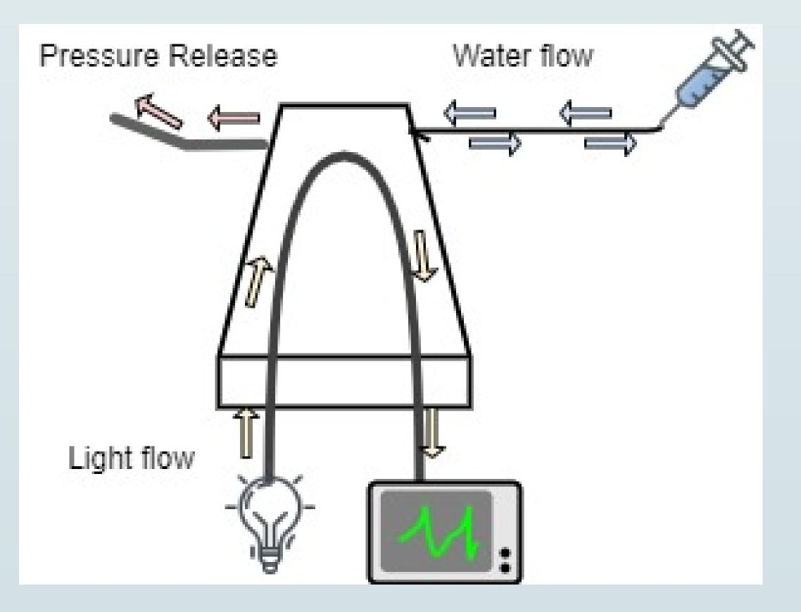
A small tube was inserted to release the pressure as water flows into the fluidic channel The sensor is connected to a light source and an Optical Spectrum Analyzer.
