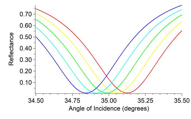
(E) 1.0-HD) 0.8-0.6-0.0-0.0-1.318 1.319 1.320 1.321 1.322 Refractive Index of Cover Layer We then slightly varied the refractive index of the cover layer, resulting in a shift in the resonance angle.
